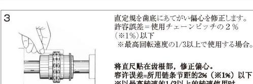
Check the parallel misalignment by measuring the gap between the bottom teeth of the two sprockets with a thickness gage or any proper measuring tools.
