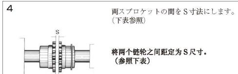
Adjust the sprockets for the proper gap "S" as shown below.
